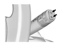
Press the upper or lower portion of the button to control the rear wiper and rear wiper delay.
